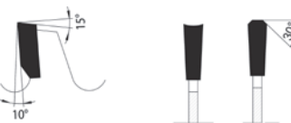
Hohlzahn-Dach-Flach Hollow inverted V/flat tooth
