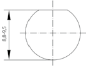
Spannfläche am Bohrer Clamping surface on drill
